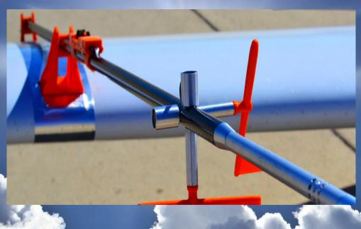
EURO FLIGHT TEST transforms any light aircraft into a test aircraft. By using a portable NON INTRUSIVE FLIGHT TEST INSTRUMENTATION system with WLAN capability, flight test data can be analyzed by a test engineer in real time aboard the test aircraft
